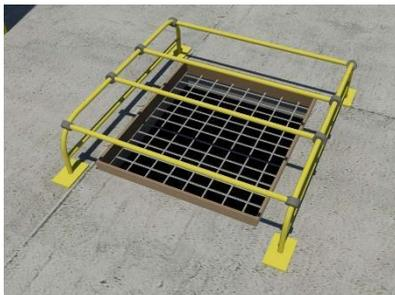
Fall protection covers are installed over openings and holes (like skylights) to prevent falls. They are usually made of timber, metal or wire mesh. They should be fixed in place and strong enough to stop a person falling through.
