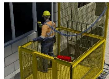
Forklift work platforms are designed to lift people with a forklift. Never stand on a pallet or the forks.
